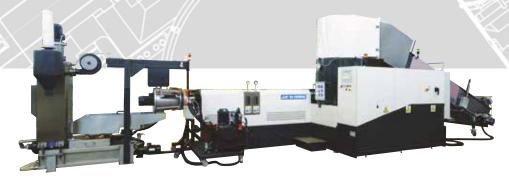
Every plant is custom designed and built to offer the best performance and yield the best quality granule that are distinguished by dimensional uniformity and absence of defects such as "air bubbles" or "twins".
