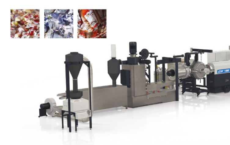
The TANDEM technology applied to the recycling of heavily printed, contaminated and high humidity plastic materials guarantees the excellent quality of the granule with a notable energy savings in comparison with conventional recycling systems that foresee the re-extrusion of the material.
